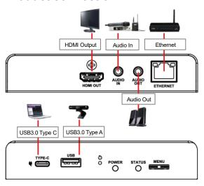
\*Decoder supports PoE (IEEE 802.3af) network switches or USB-C power supply
